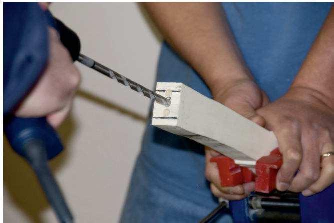
Using a drill to open up the tang hole.
