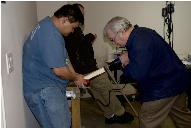
Using a drill to open up the tang hole.
