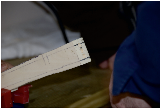
The three completed pilot holes.
